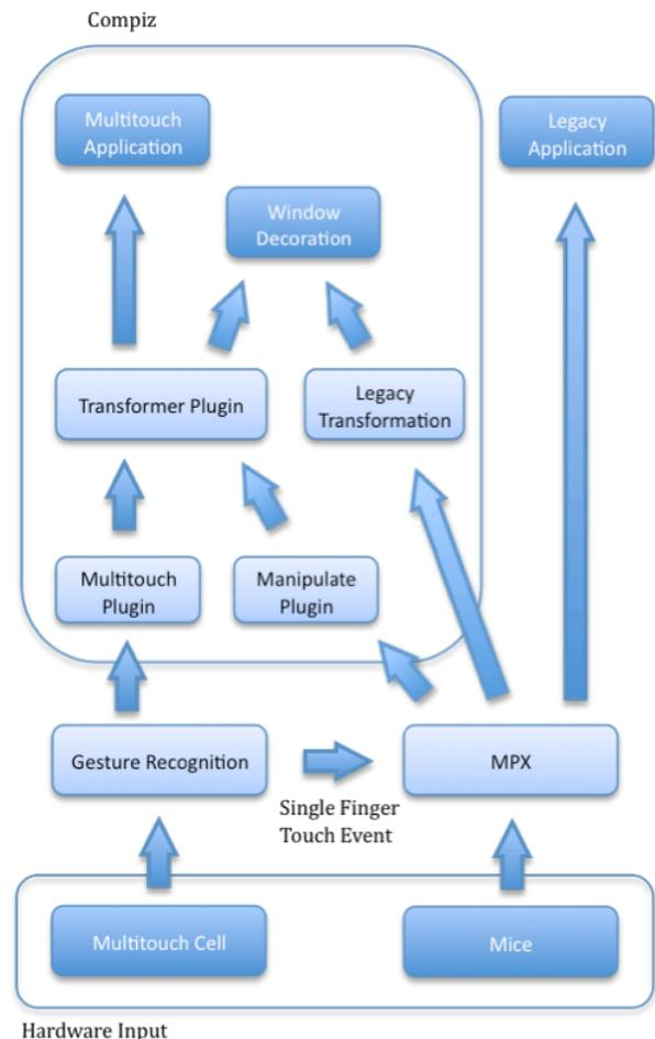
**Figure 3.** Our implementation of the unified software architecture.
