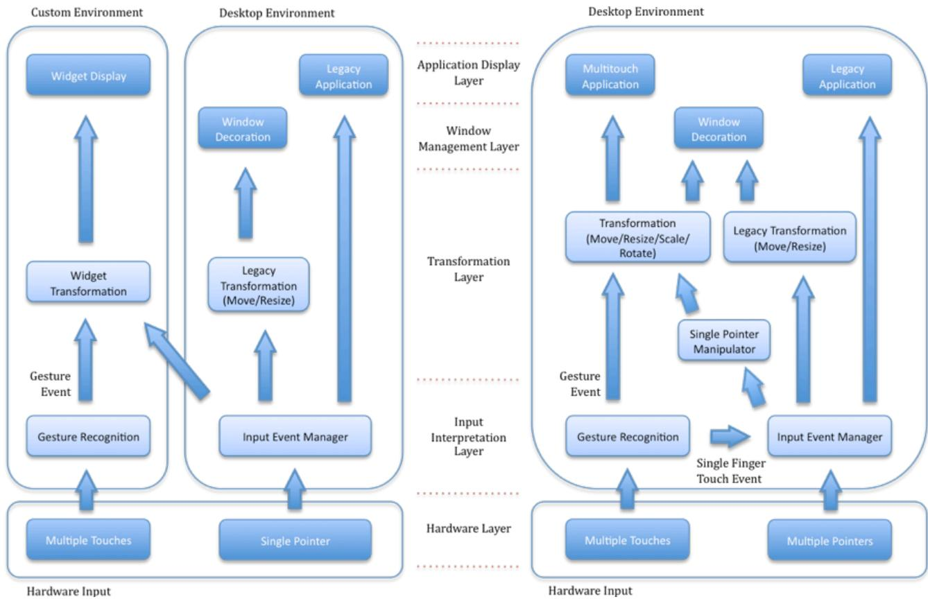
**Figure 1. Left: Current architecture separates custom multi-touch aware environment and the underlying desktop. Right: Unified architecture for simultaneous multi-touch and multi-pointer input on the desktop environment.**
