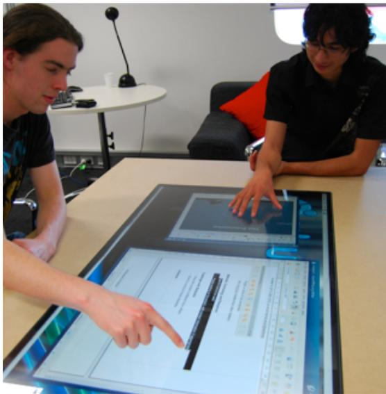
**Figure 2.** A user using a single pointer via touch, and another using a five-finger rotation gesture.
