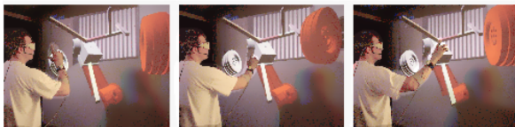
Figure 11: Rotating an object using a mimetic 8 gesture. The user says “...and turn it this way...” and describes the desired manipulation in parallel. The system continuously converts the unprecise arm movement into a precise object manipulation.
