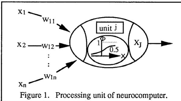
Figure 1. Processing unit of neurocomputer.
